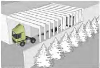
Figure 5.2 (6). Screened loading area.
