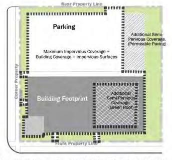
Figure 5.2 (3). Maximum Impervious & Additional Semi-Pervious Coverage.
