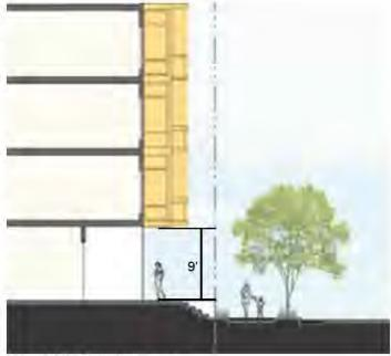
Figure 5.1 (1). Projection Clearance.
