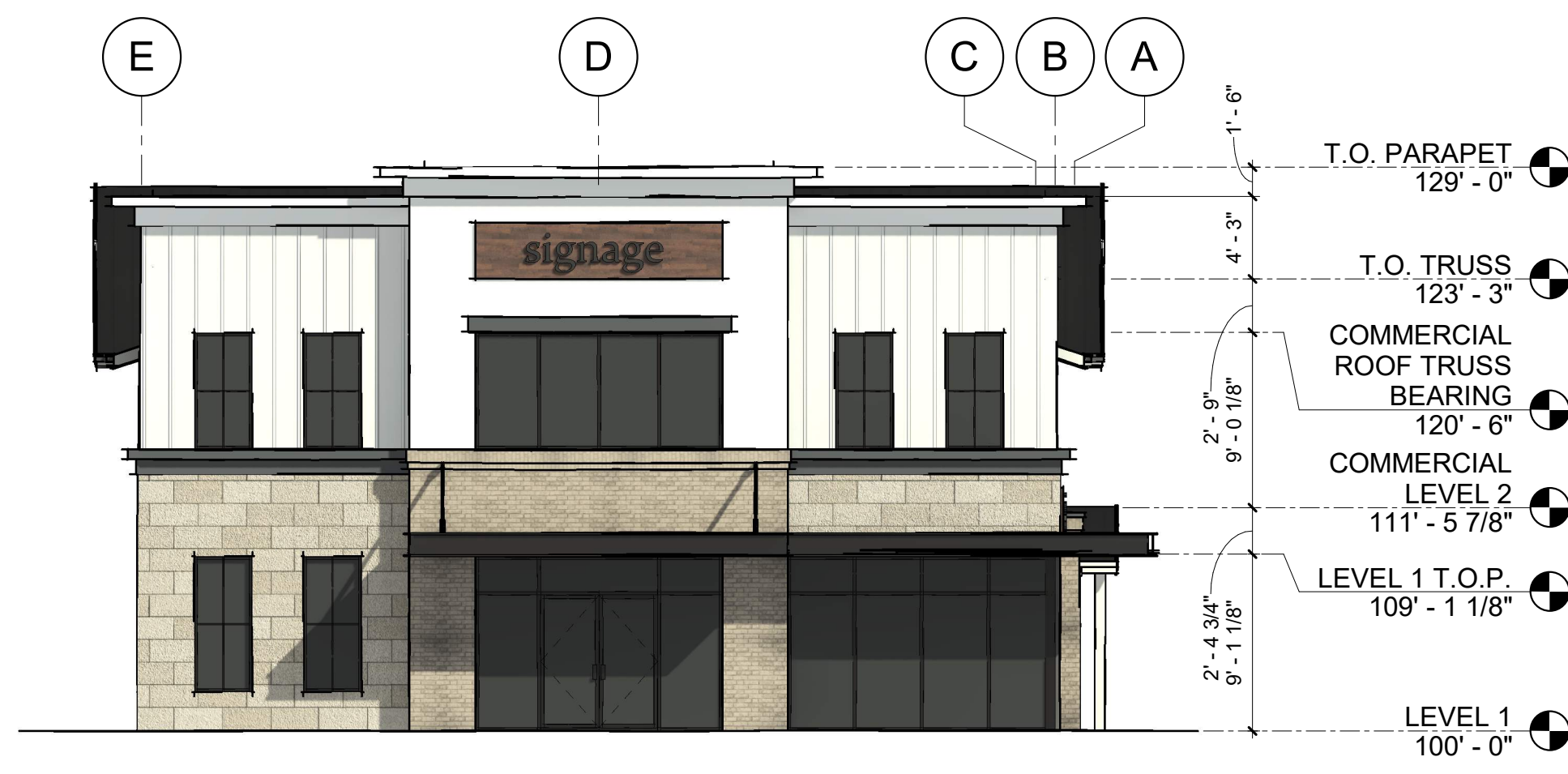
C3 WEST EXTERIOR ELEVATION 1/8" = 1'-0"
