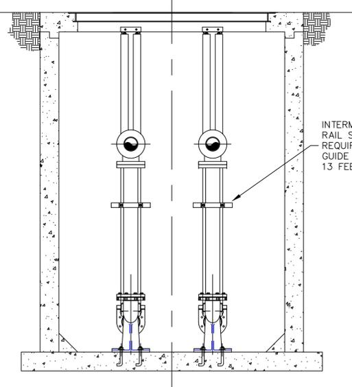
INTERMEDIATE GUIDE RAIL SUPPORT REQUIRED FOR GUIDE RAILS OVER 13 FEET LONG.
