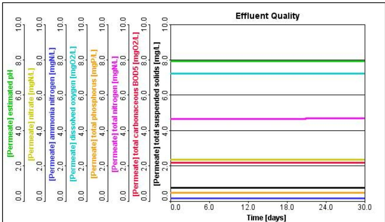
Figure 3.7: MLE MDF Effluent Quality at RAS = 2Q and DO = 0.5 mg/L
