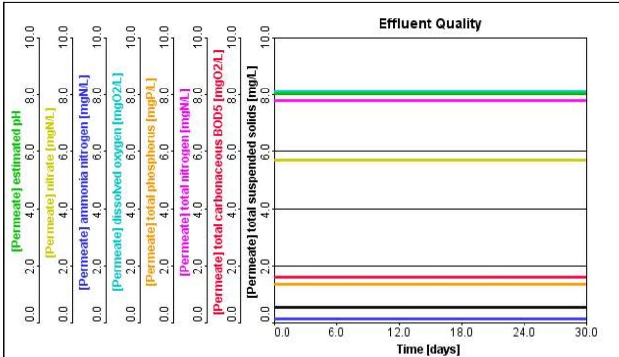
Figure 3.4: MLE AAF Effluent Quality at RAS = 2Q and DO = 1 mg/L
