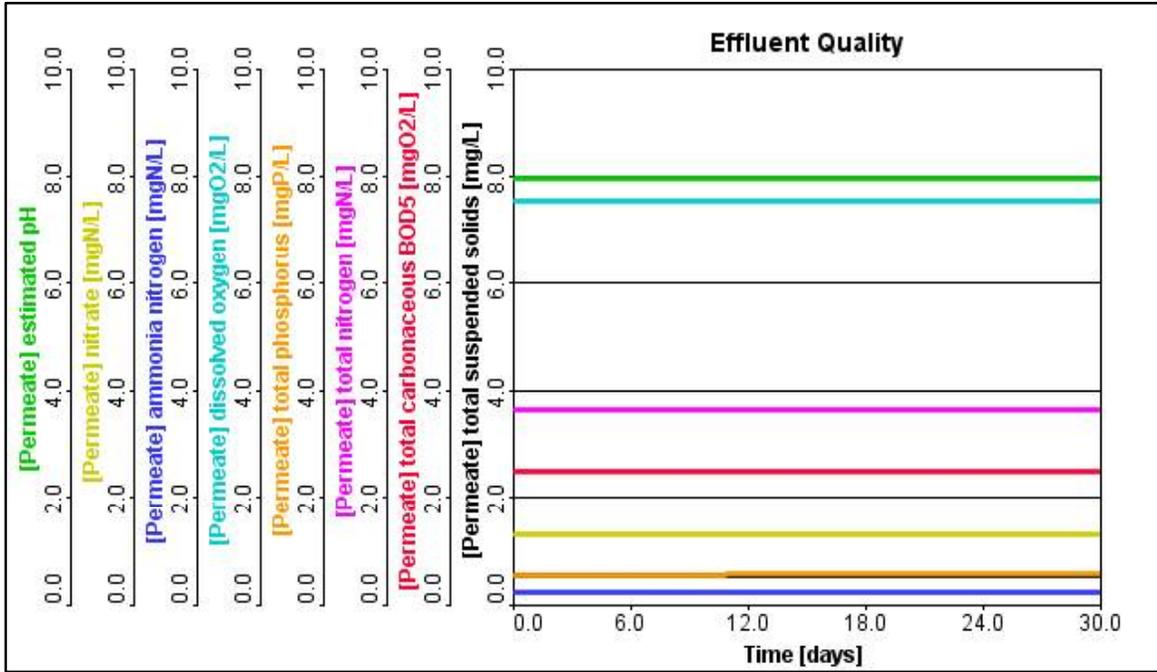
Figure 4.4: Bardenpho AAF Effluent Quality at internal recycle rate = 1Q
