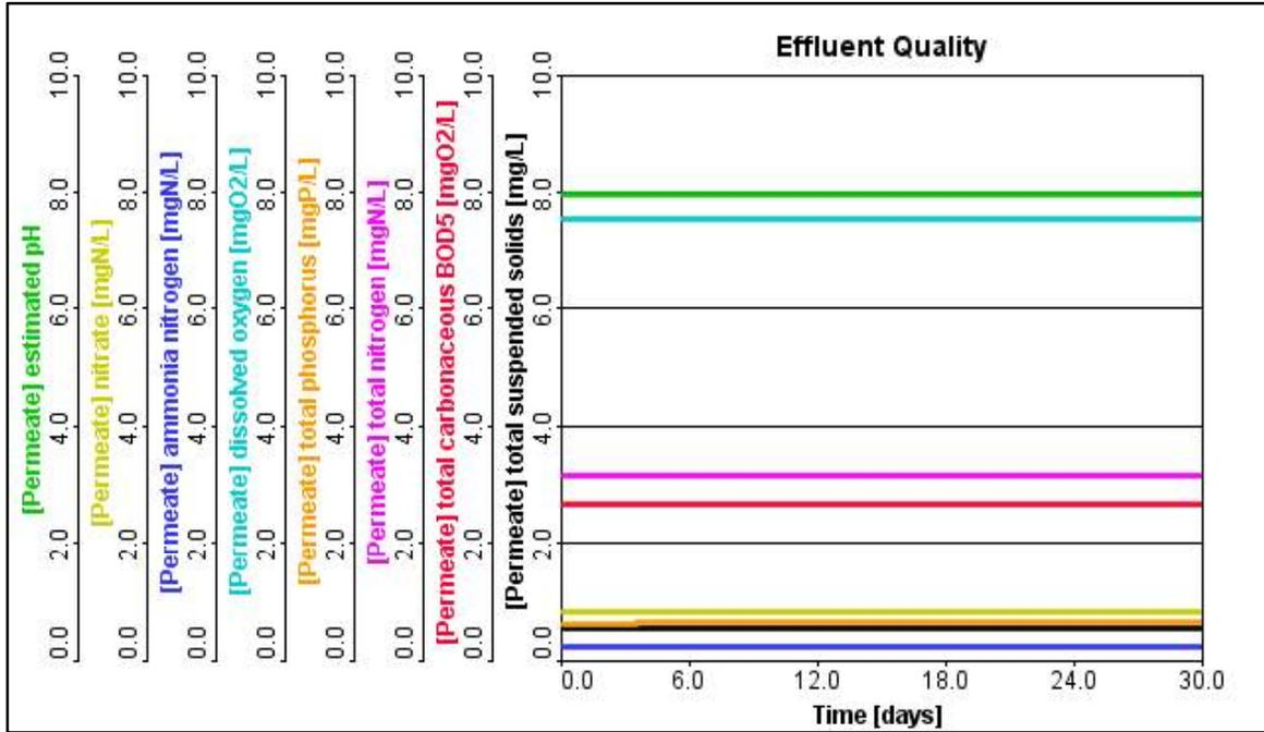
Figure 4.2: Bardenpho AAF Effluent Quality at internal recycle rate = 4Q
