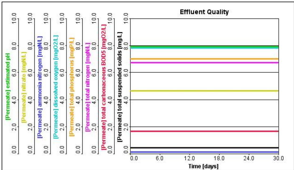
Figure 3.2: MLE AAF Effluent Quality at RAS = 4Q and DO = 2 mg/L
