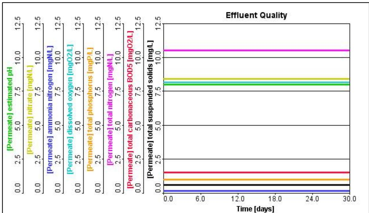
Figure 3.5: MLE AAF Effluent Quality at RAS = 1Q and DO = 1 mg/L
