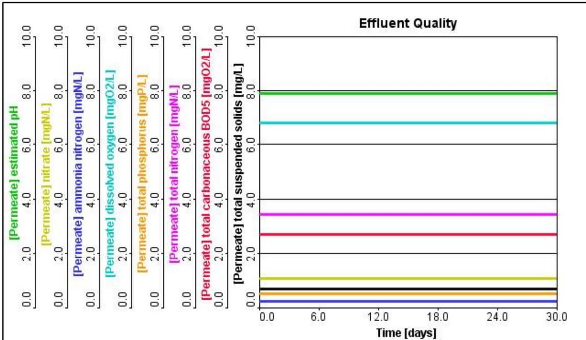
Figure 4.5: Bardenpho MDF Effluent Quality at internal recycle rate = 2Q
