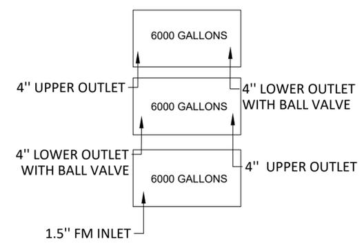
**18000 GAL SLUDGE STORAGE SCHEMATIC
