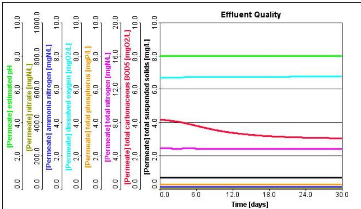
Figure 5.4: Johannesburg AAF Effluent Quality at DO = 2 mg/L, Methanol Feed = 1.25 gph
