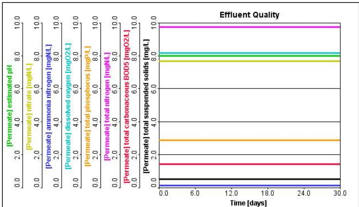
Figure 3.3: MLE AAF Effluent Quality at RAS = 2Q and DO = 2 mg/L
