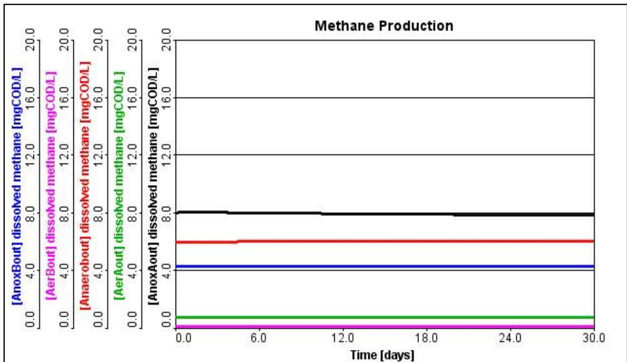
Figure 5.5: Johannesburg AAF Methane Production at DO = 2 mg/L, Methanol Feed = 1.25 gph
