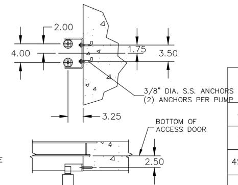
UPPER GUIDE RAIL BRACKET MOUNTING DETAIL
