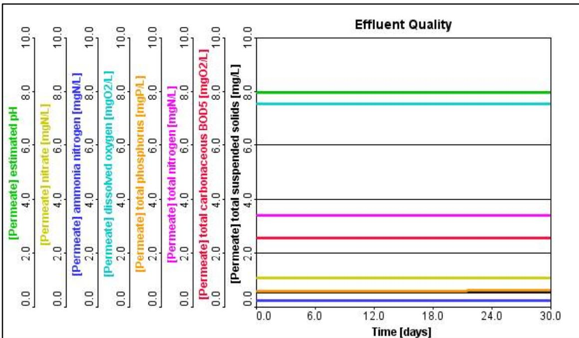
Figure 4.3: Bardenpho AAF Effluent Quality at internal recycle rate = 2Q
