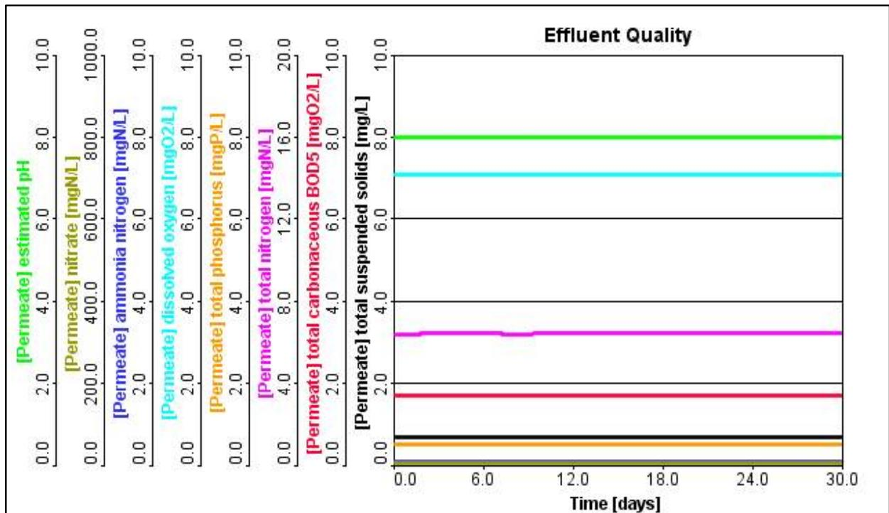
Figure 5.3: Johannesburg AAF Effluent Quality at DO = 2 mg/L, Methanol Feed = 0.25 gph
