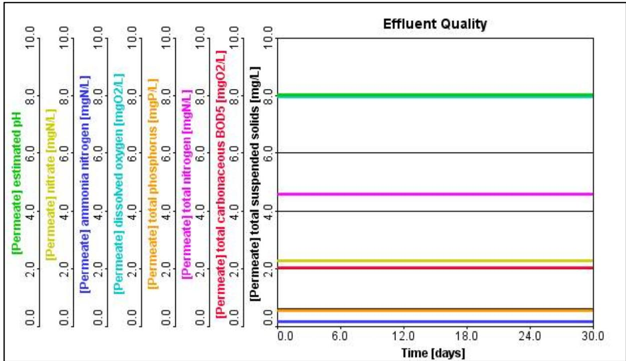
Figure 3.6: MLE AAF Effluent Quality at RAS=2Q and DO=0.5 mg/L
