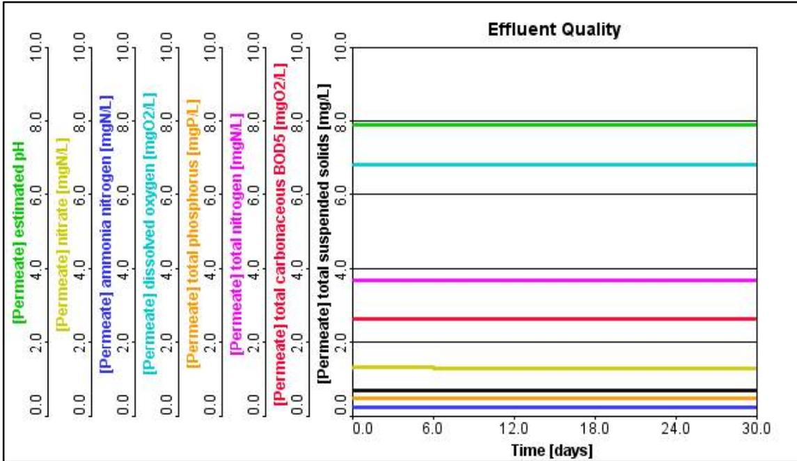
Figure 4.6: Bardenpho MDF Effluent Quality at internal recycle rate = 1Q
