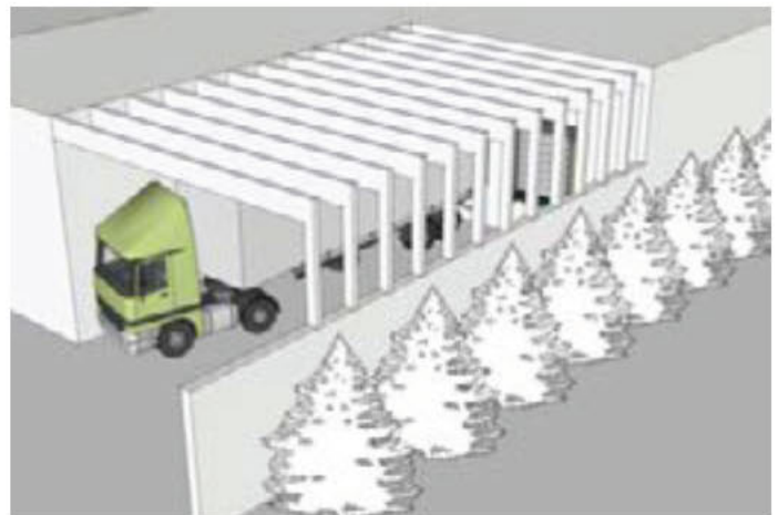
Figure 5.2 (6). Screened loading area.
