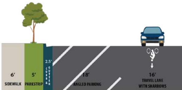
Figure 44: Half street cross-section of a road with angle parking and marked shared roadway.
