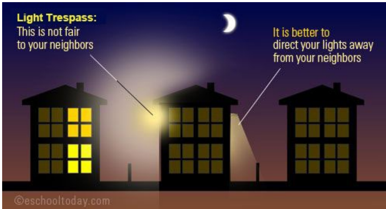
Figure 09: Light Trespass Compared to Adequate Shielding (adapted from E School Today 2023 https://eschooltoday.com/learn/types-of-light-pollution/ )
