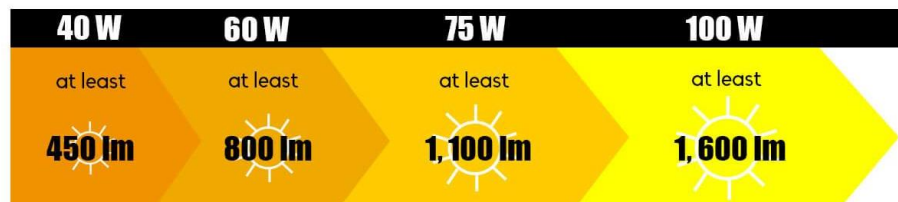
Figure 05: Watts to Lumens Relationship (adapted from Standard Products Inc 2023 https://www.standardpro.com/how-to-measure-light/ )
