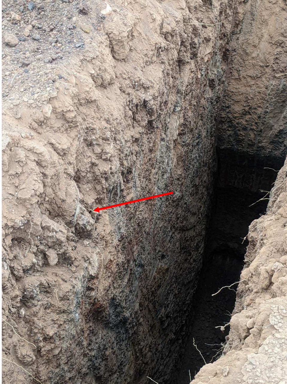
Photo No. 7, View of Test Pit TP-1, Arrow indicates approximate boundary or top of mudstone/blue clay
