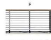
F STEEL GUARDRAIL WITH IPE WOOD TOP RAIL
