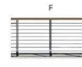
F STEEL GUARDRAIL WITH IPE WOOD TOP RAIL
