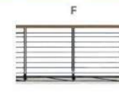
STEEL GUARDRAIL WITH IPE WOOD TOP RAIL
