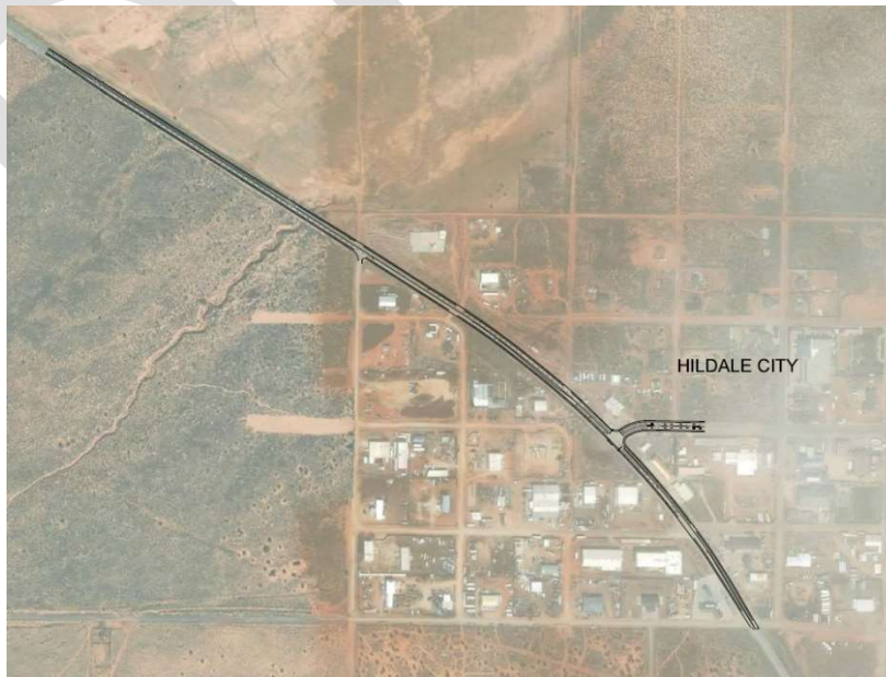
Figure 2 Concept of Intersection Widening
