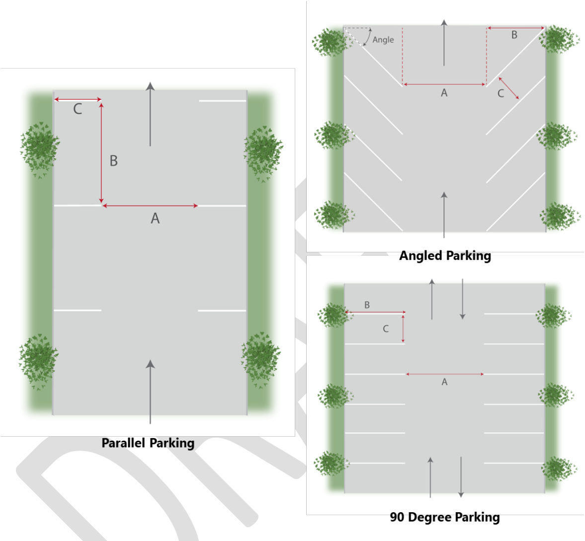
Figure 19.49.030: Parking Space and Aisle Dimensions.
