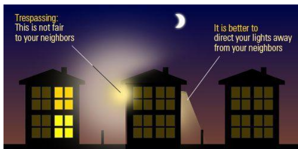
Figure 09: Light Trespass Compared to Adequate Shielding
