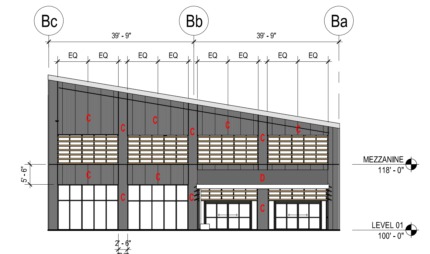
C5 PEMB - NEW EXTERIOR ELEVATION - SOUTH ENTRY 1/16" = 1'-0"
