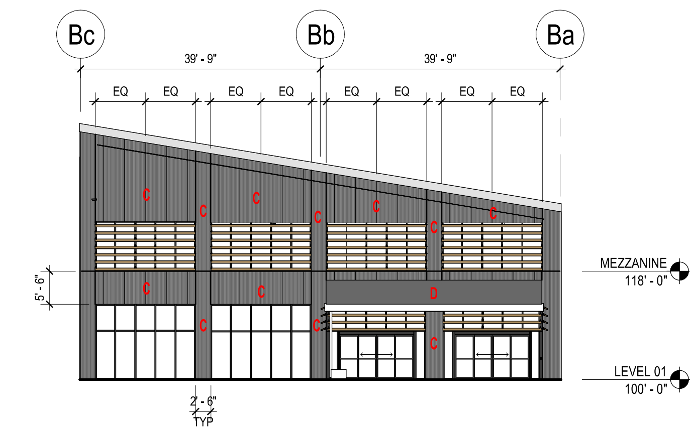
C5 PEMB - NEW EXTERIOR ELEVATION - SOUTH ENTRY 1/16" = 1'-0"
