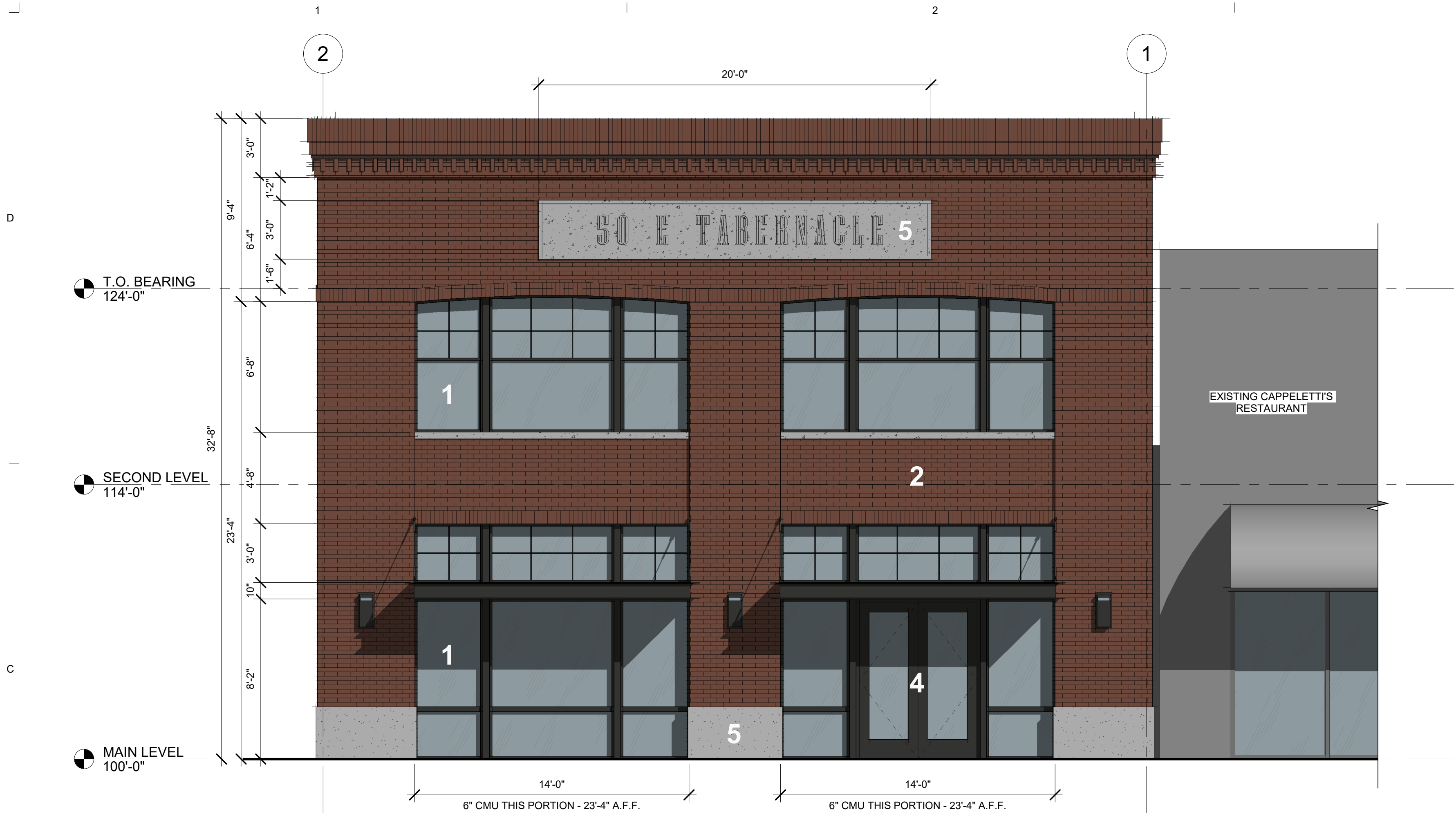
C1 NORTH EXTERIOR ELEVATION 1/4" = 1'-0"
