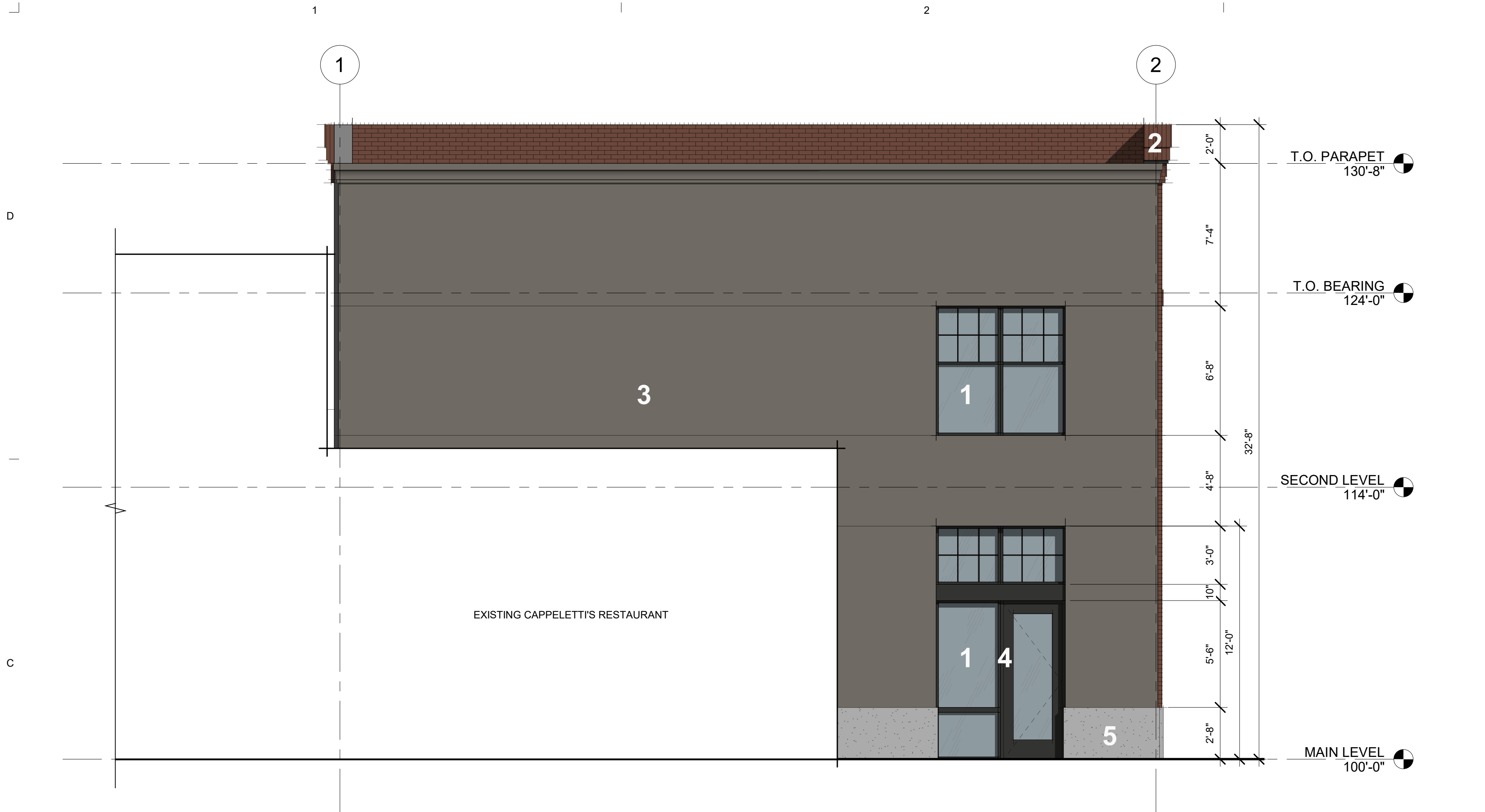
C1 SOUTH EXTERIOR ELEVATION 1/4" = 1'-0"
