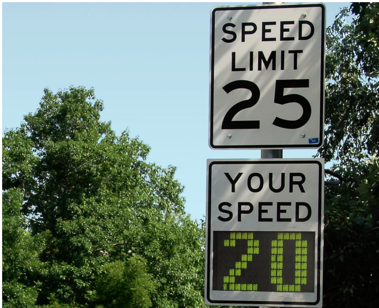
Figure 1: Typical flashing speed sign configuration
