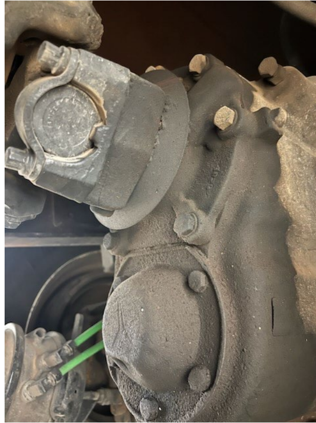
Pinion Seal Leak
