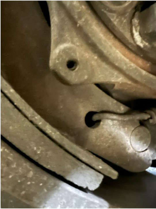
Brake Shoe Separating from Backing
