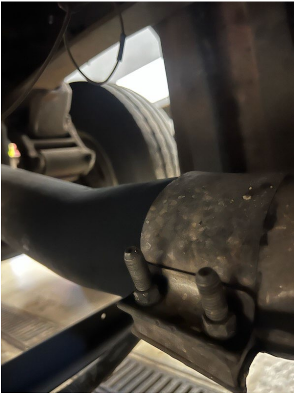
Exhaust Leak under Cab
