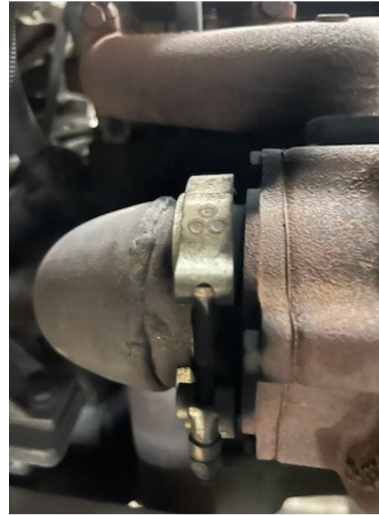
Exhaust Leak at Turbo
