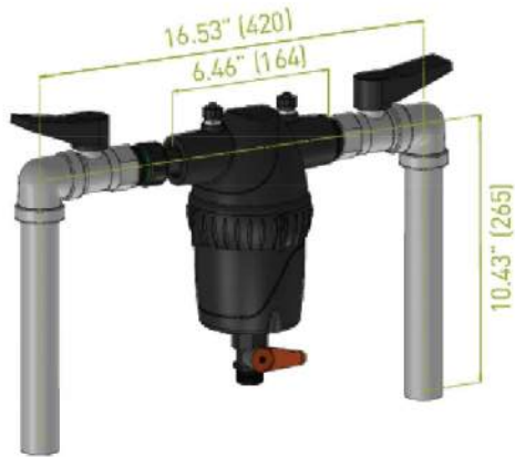
2. DETAIL - 1" AMIAD FILTER W/ BRUSHAWAY ASSEMBLY NOT TO SCALE
