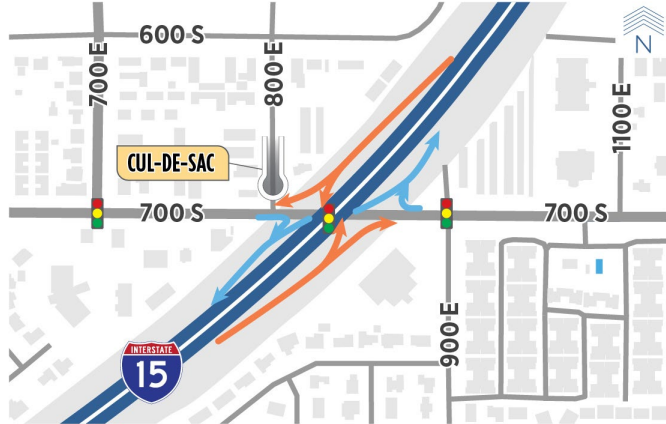
Single Point Urban Interchange (SPUI)
