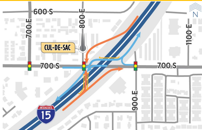
Offset SPUI w/ EB to NB Crossover
