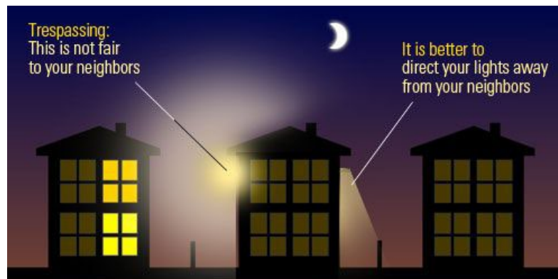
Figure XX: Light trespass Compared to Adequate Shielding
