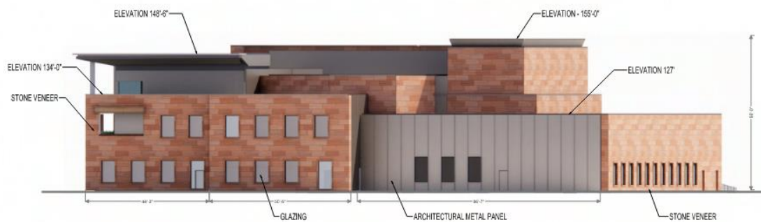
EAST ELEVATION - SHARED DOTERRA MOB PLAZA
