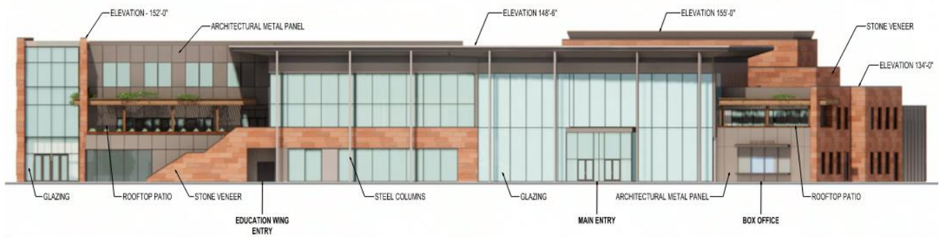
SOUTH ELEVATION - MAIN ENTRY
