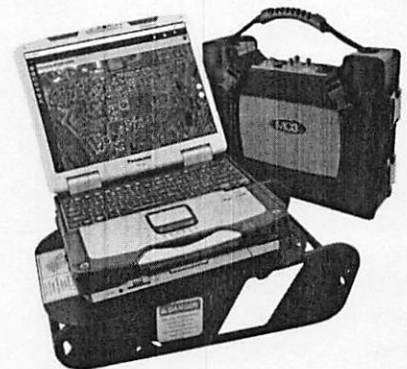
Itron MC3 Radio (actual size: 13" W x 11.25" L x 2.75" H)
