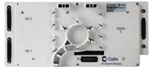
Figure 13. RSX3001 switch module
