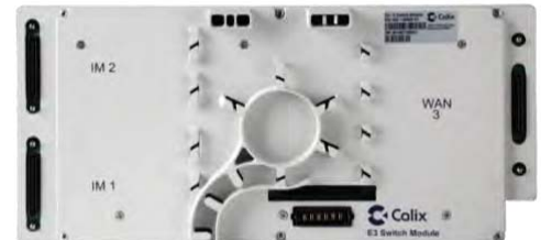
Figure 15. RSX3101E 10G EPON switch module
