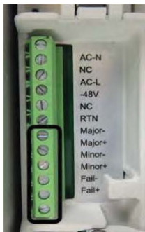
Figure 17. Figure 15 - E3-2 Terminal Block with Environmental Alarm Contacts
