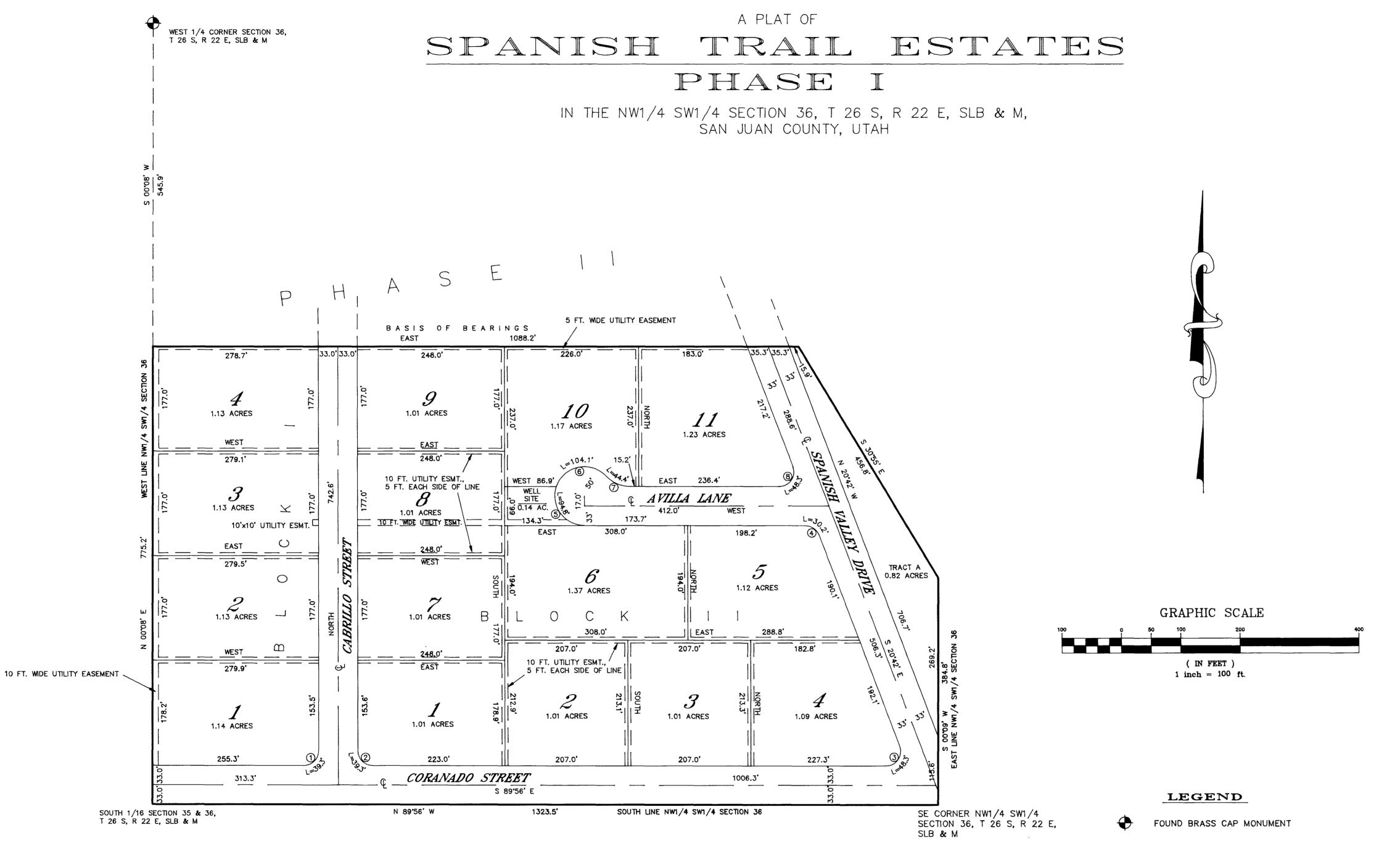
1. SET 5/8" REBAR WITH PLASTIC CAP AT EACH CORNÉR AND OR CURVE POINT.
