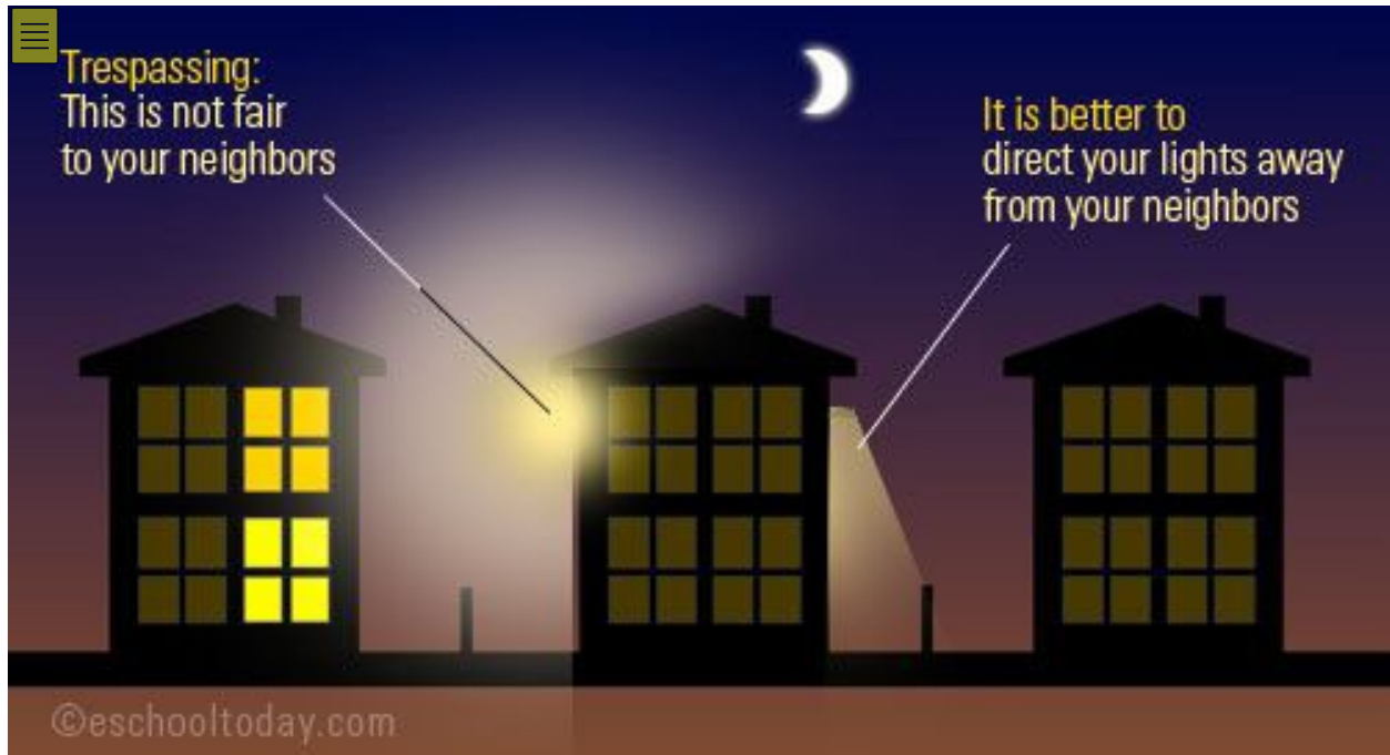
Figure 6: Light Intrusion Compared to Adequate Shielding
