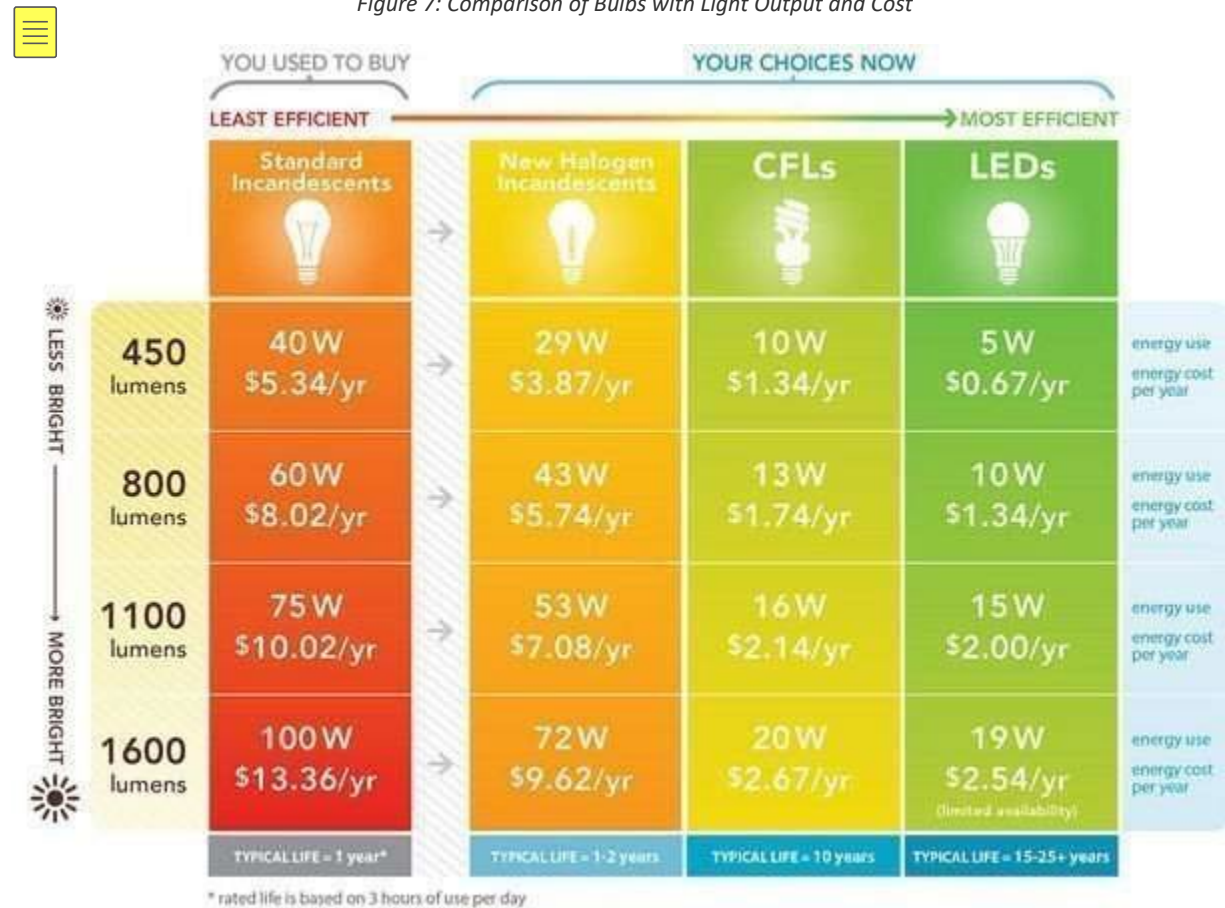
Figure 7: Comparison of Bulbs with Light Output and Cost
