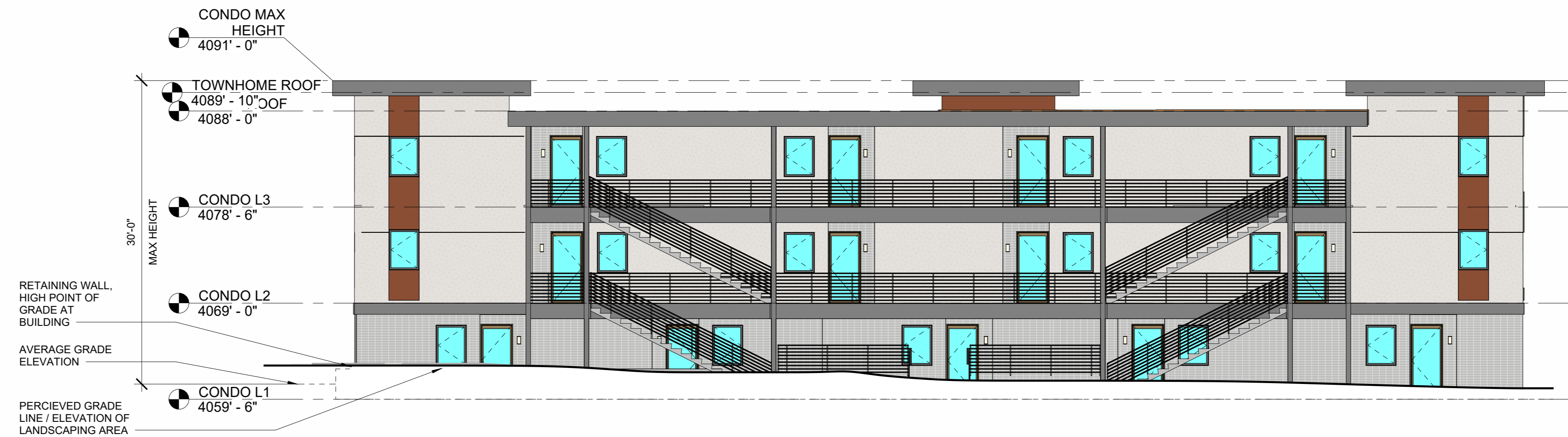
5 CONDO ELEVATION - NORTH 1/8" = 1'-0"
