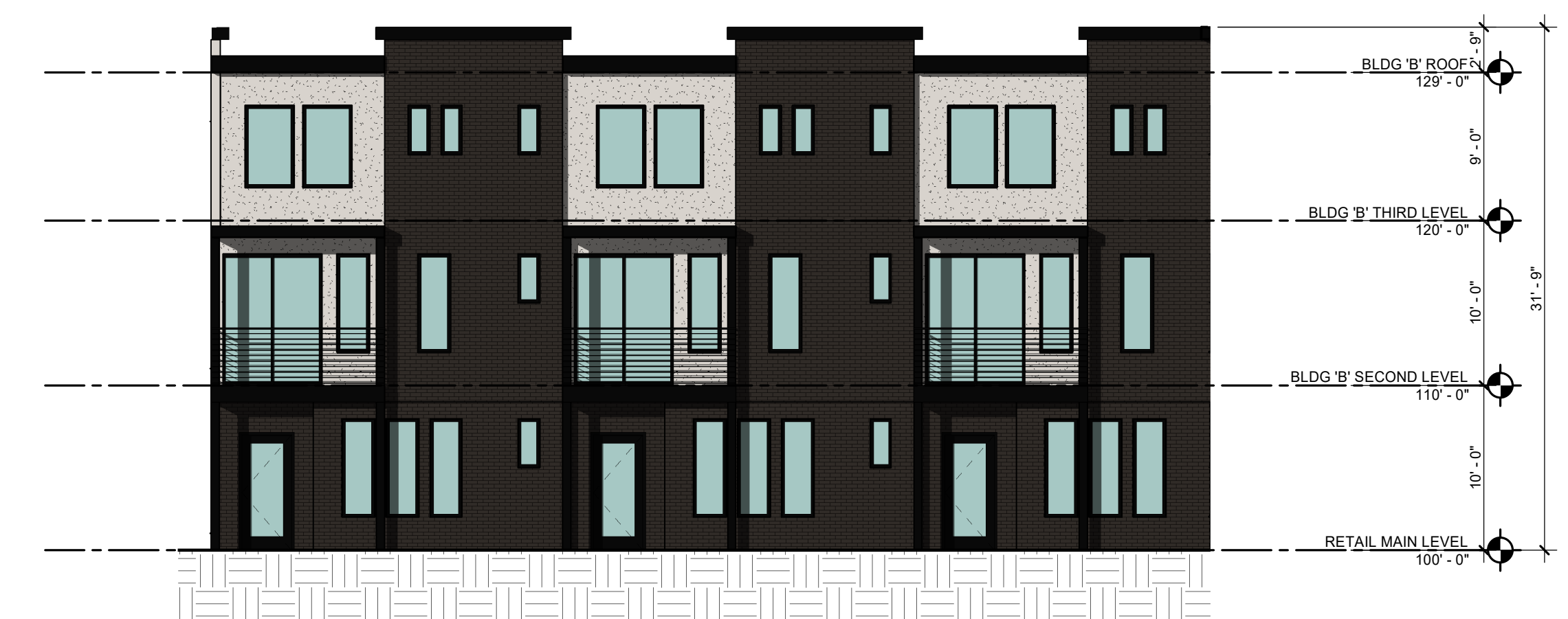
02 WEST ELEVATION - BUILDING TYPE 'E' 1/8" = 1'-0"
