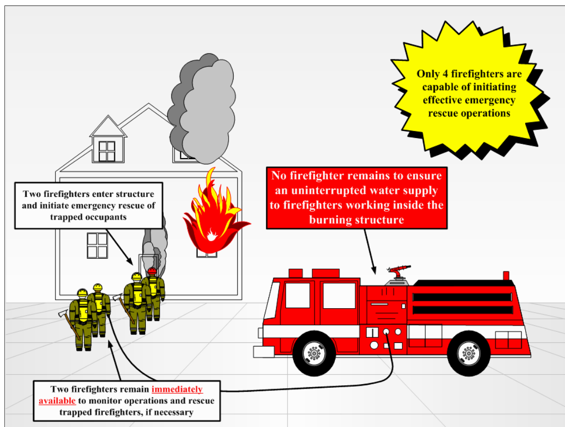
FIGURE 5-2: Two-In/Two-Out Interior Firefighting Model*
