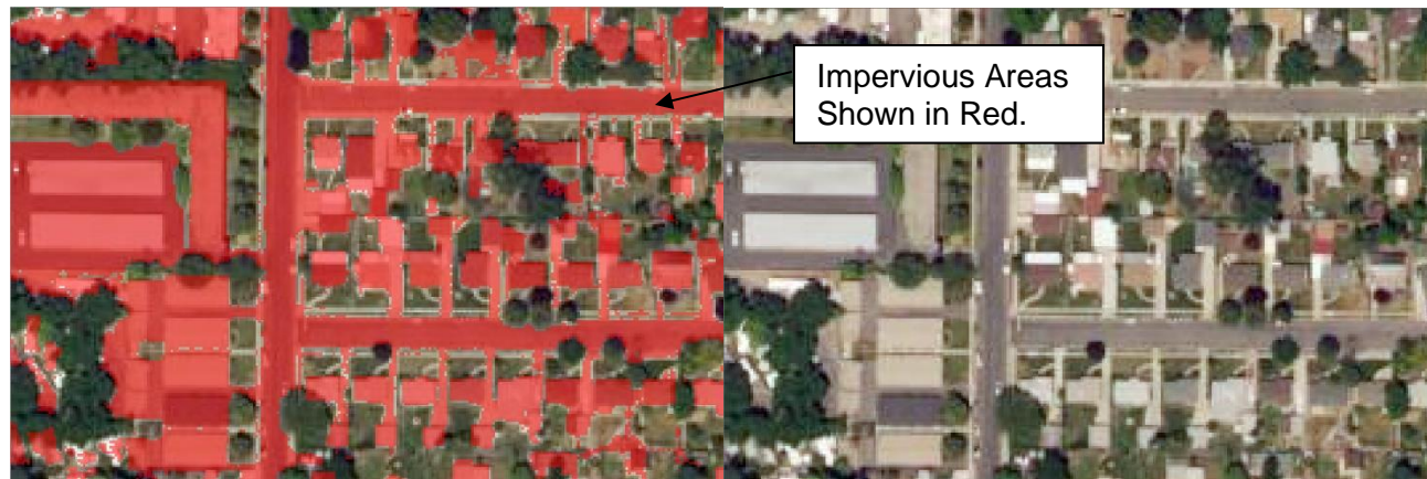
FIGURE 1. EXAMPLE OF IMPERVIOUS AREA DEFINED BY REMOTE SENSING DATA
