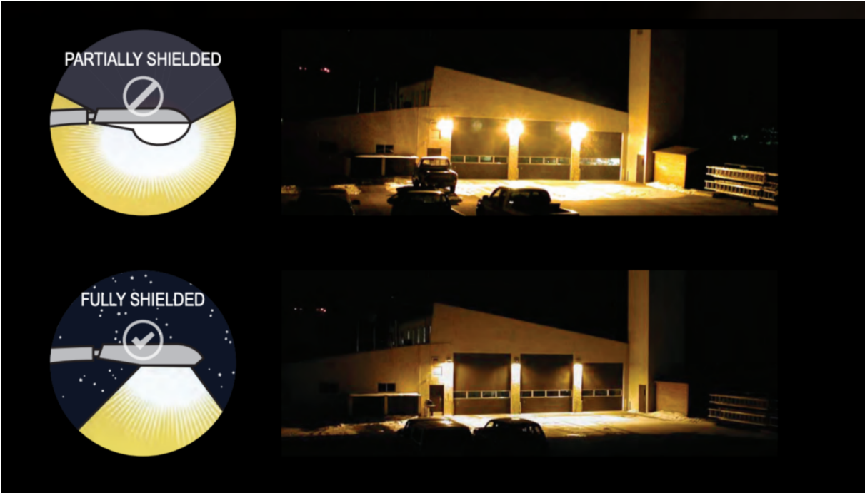
Figure 7. Fully shielded vs. partially shielded light fixtures
