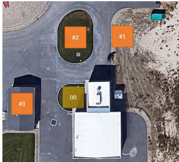
Figure 4: Alternative Grit Washing Building locations (orange) compared to original planned location northwest corner of East Headworks (yellow). Squares shown are approximately 30 feet by 30 feet.
