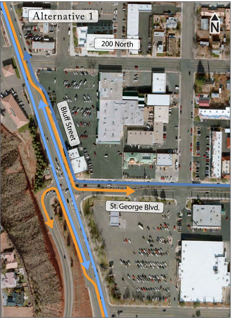
Continuous Flow Intersection
