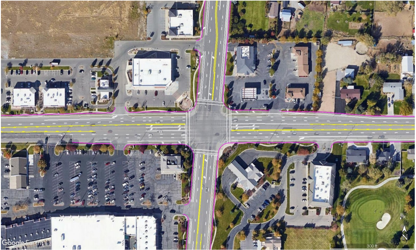
Figure 13. 5300 West (S.R. 74) Intersection Concept Design
