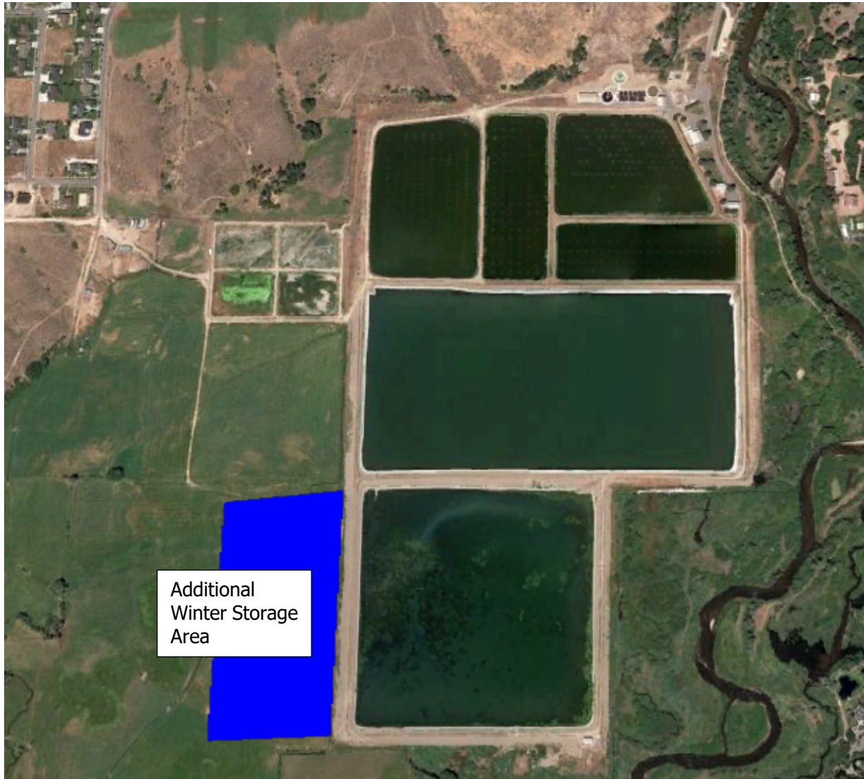
Figure 3 Additional Storage Required
