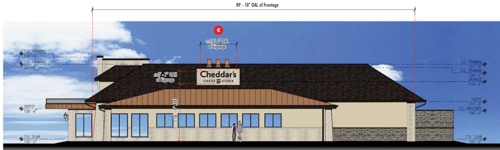
2 SOUTH ELEVATION (FACES RIVERDALE ROAD) SIGN SQUARE FOOTAGE FOR ELEVATION = 35.90 SQ. FT. (MAX ALLOWED @ 3 SF PER 1 FT. LINEAR, 248 SF) SCALE: 3/32" = 1' - 0"
