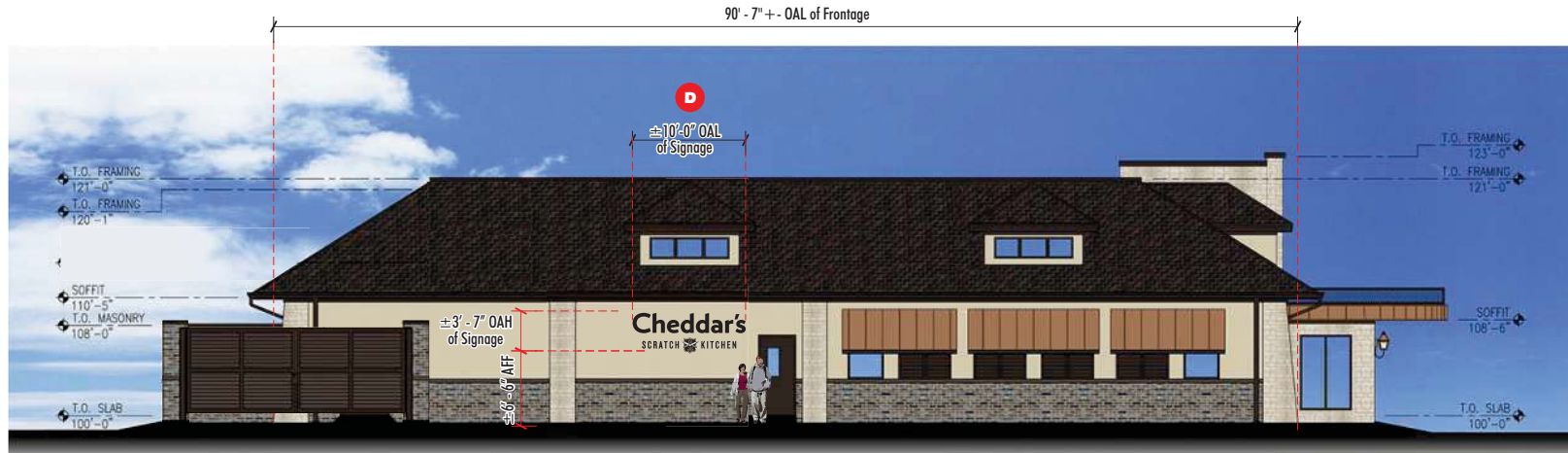
2 NORTH ELEVATION (SHOPPING CENTER) SIGN SQUARE FOOTAGE FOR ELEVATION = 35.90 SQ. FT. (MAX ALLOWED @ 3 SF PER 1 FT. LINEAR, 248 SF) SCALE: 3/32" = 1' - 0"
