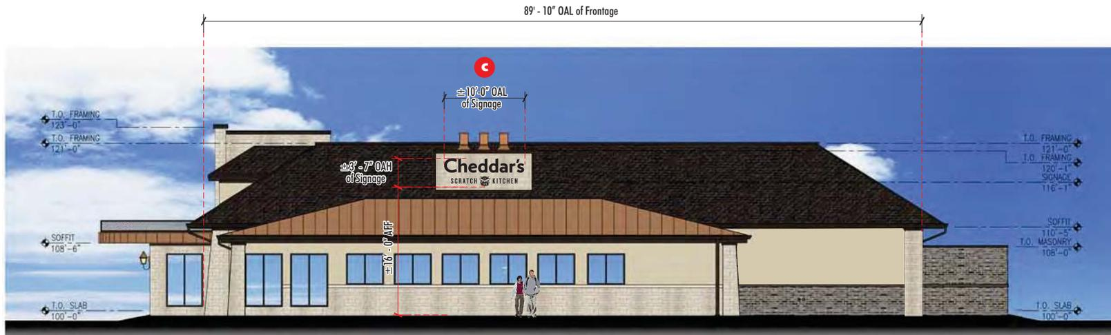
**2** SOUTH ELEVATION (FACES RIVERDALE ROAD) SIGN SQUARE FOOTAGE FOR ELEVATION = 35.90 SQ. FT. (MAX ALLOWED @ 3 SF PER 1 FT. LINEAR, 248 SF)
