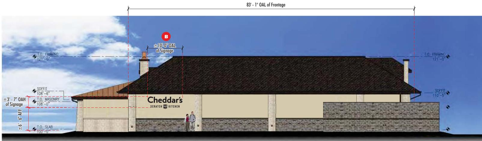
**1** EAST ELEVATION (FACES ENTRANCE INTO SHOPPING CENTER) SIGN SQUARE FOOTAGE FOR ELEVATION = 35.90 SQ. FT. (MAX ALLOWED @ 3 SF PER 1 FT. LINEAR, 248 SF)
