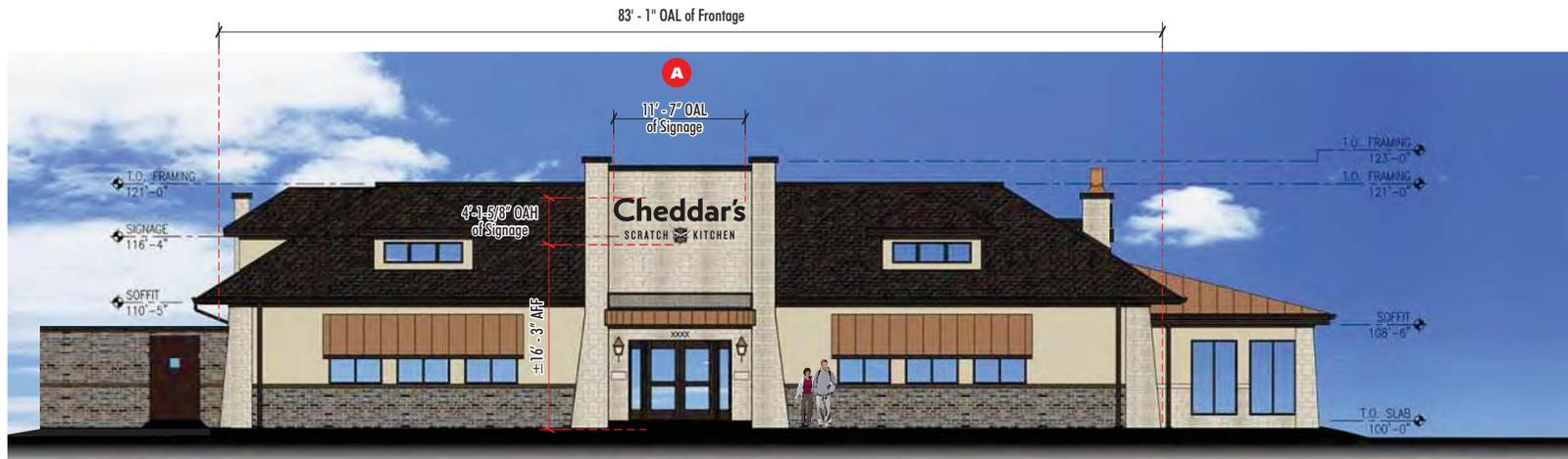
**1** WEST ELEVATION (FRONT ELEVATION) SIGN SQUARE FOOTAGE FOR ELEVATION = 47.90 SQ. FT. (MAX ALLOWED @ 3 SF PER 1 FT. LINEAR, 248 SF)
