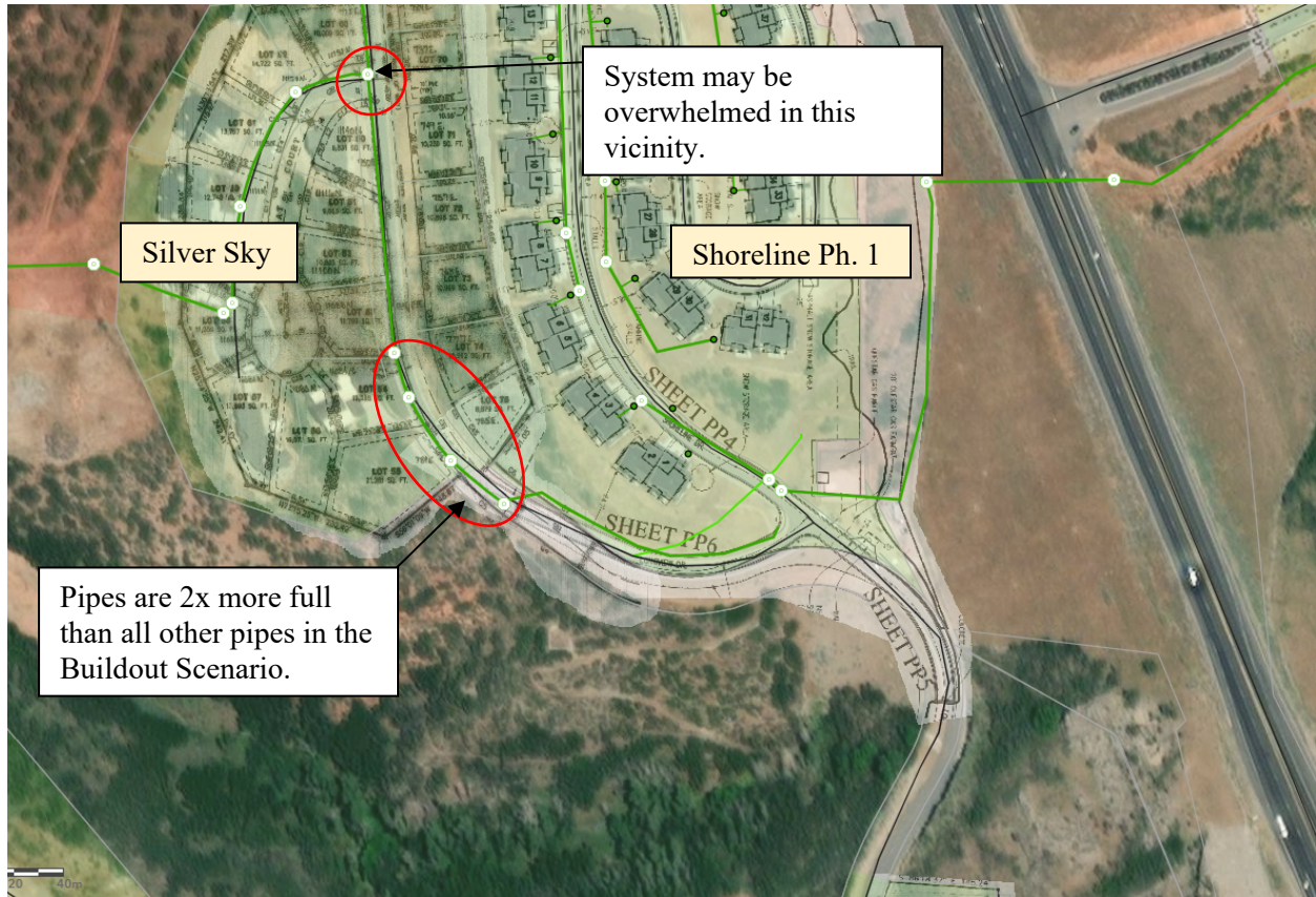
Figure 5. Pipes are Overly Full in Silver Sky
