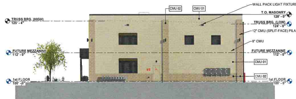
3 BUILDING A RIGHT ELEVATION 3/32" = 1'-0"
