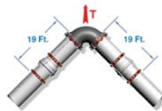
2 90° BEND RESTRAINT DETAIL N.C.E.
