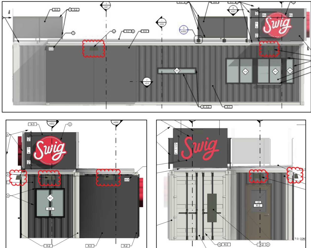
Proposed Building Elevations with Wall-Mounted Lights Marked
