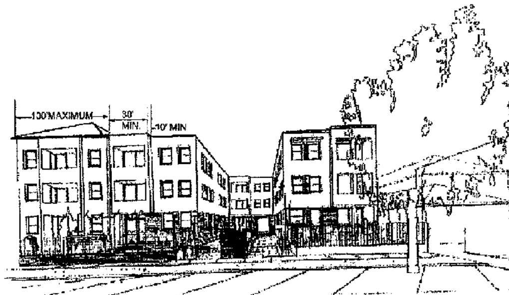
Typical Roofline Breaks
