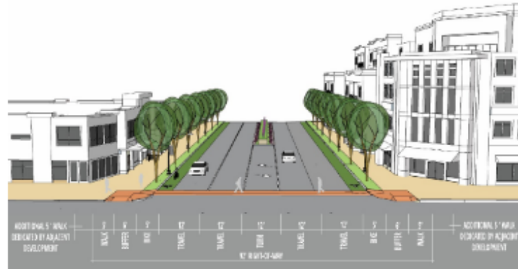
Figure 3 Typical Cross Section for Highland Drive
