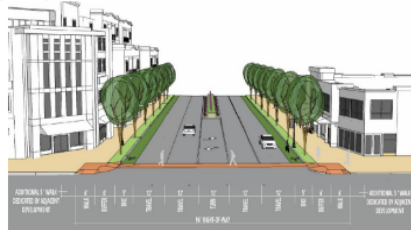
Figure 5 Typical Cross Section for 3300 South
