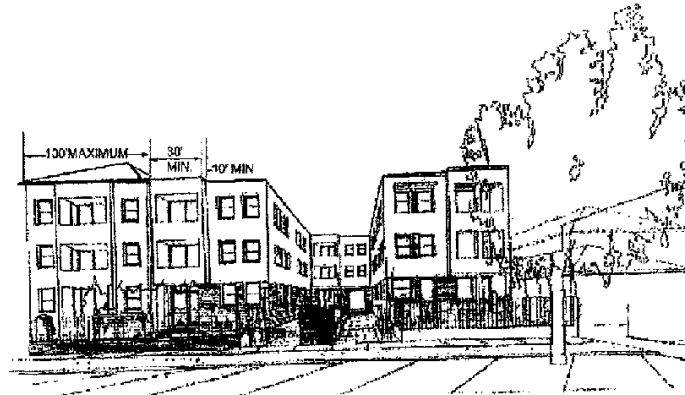
Typical Roofline Breaks
