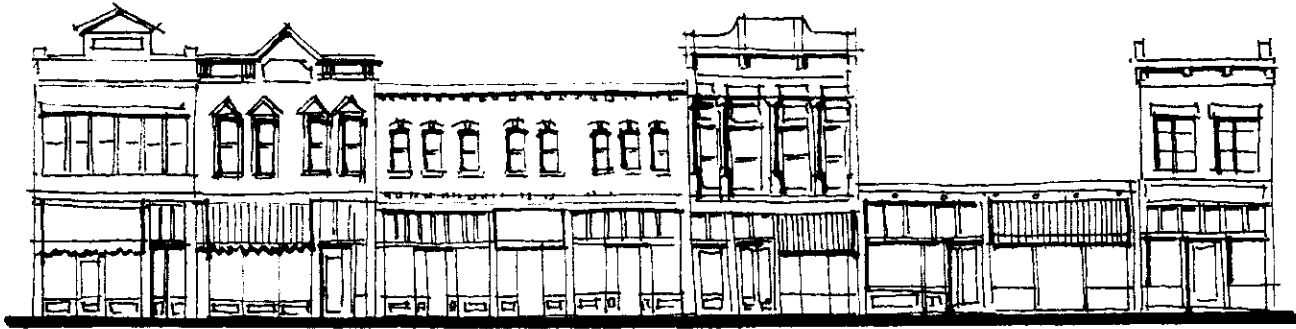
Figure 1. New Buildings should use similar orientation, setbacks, scale, height, massing, fenestration and form as surrounding historic bldgs.
