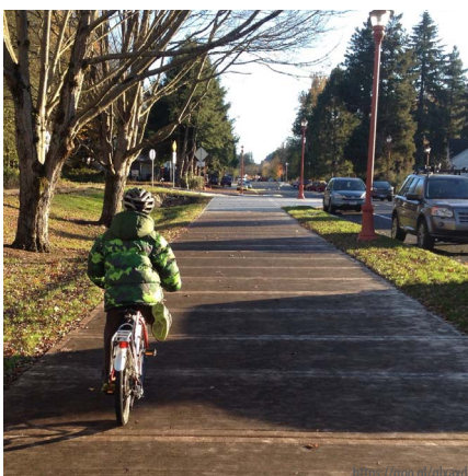
Figure 3-2. Sidewalks with widths from 5 to 10 feet provide enough room for both pedestrians and bicyclists to travel safely off-street.
