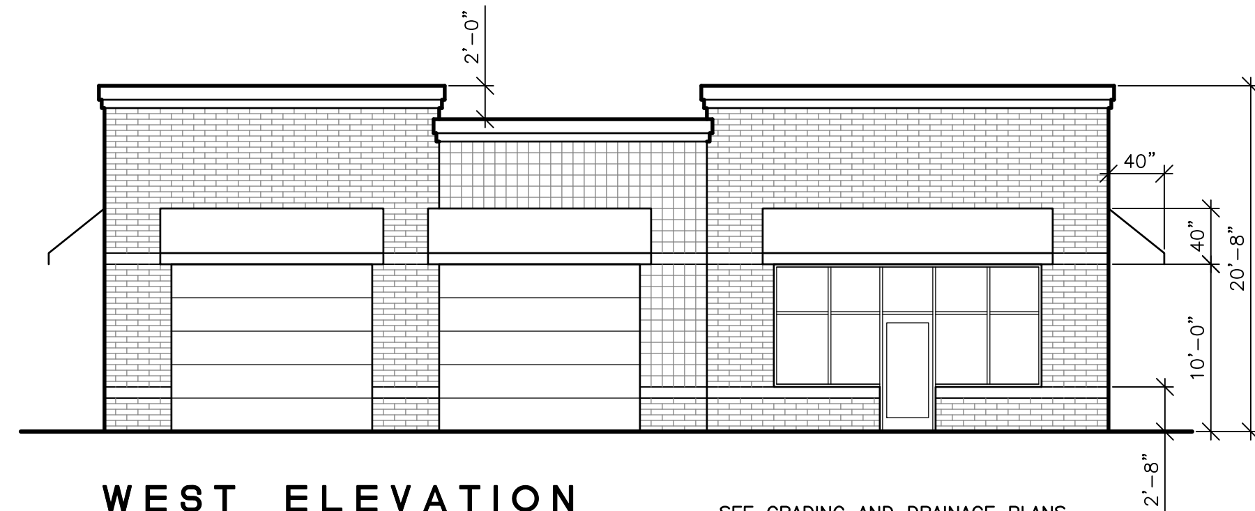
SEE GRADING AND DRAINAGE PLANS AND STRUCTURAL ENGINEER DRAWINGS PROVIDE A MIN. 30" FROST DEPTH
