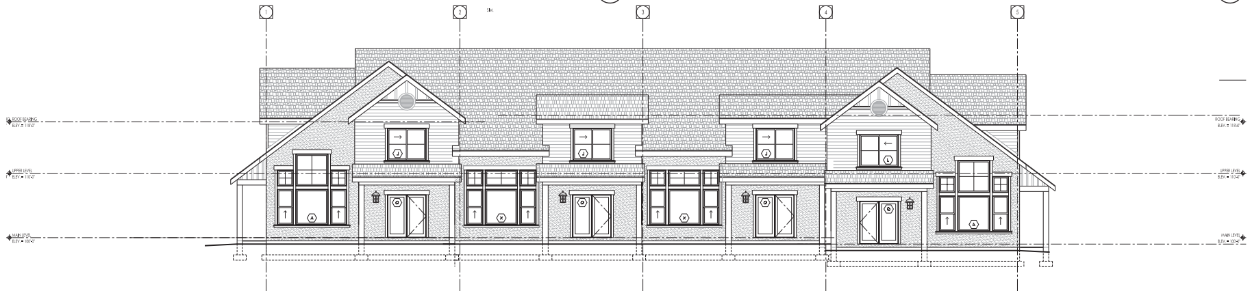
BUILDING TYPE 10 - REAR ELEVATION SCALE: 3/16" = 1'-0"
