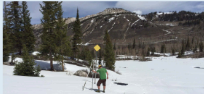
A surveyor measures the depth of the snowpack at Mt. Baldy on the Wasatch Plateau in April 2015. The map below shows the results of many years of this type of measurement. Credit: Jordan Clayton, USDA Natural Resources Conservation Service.
