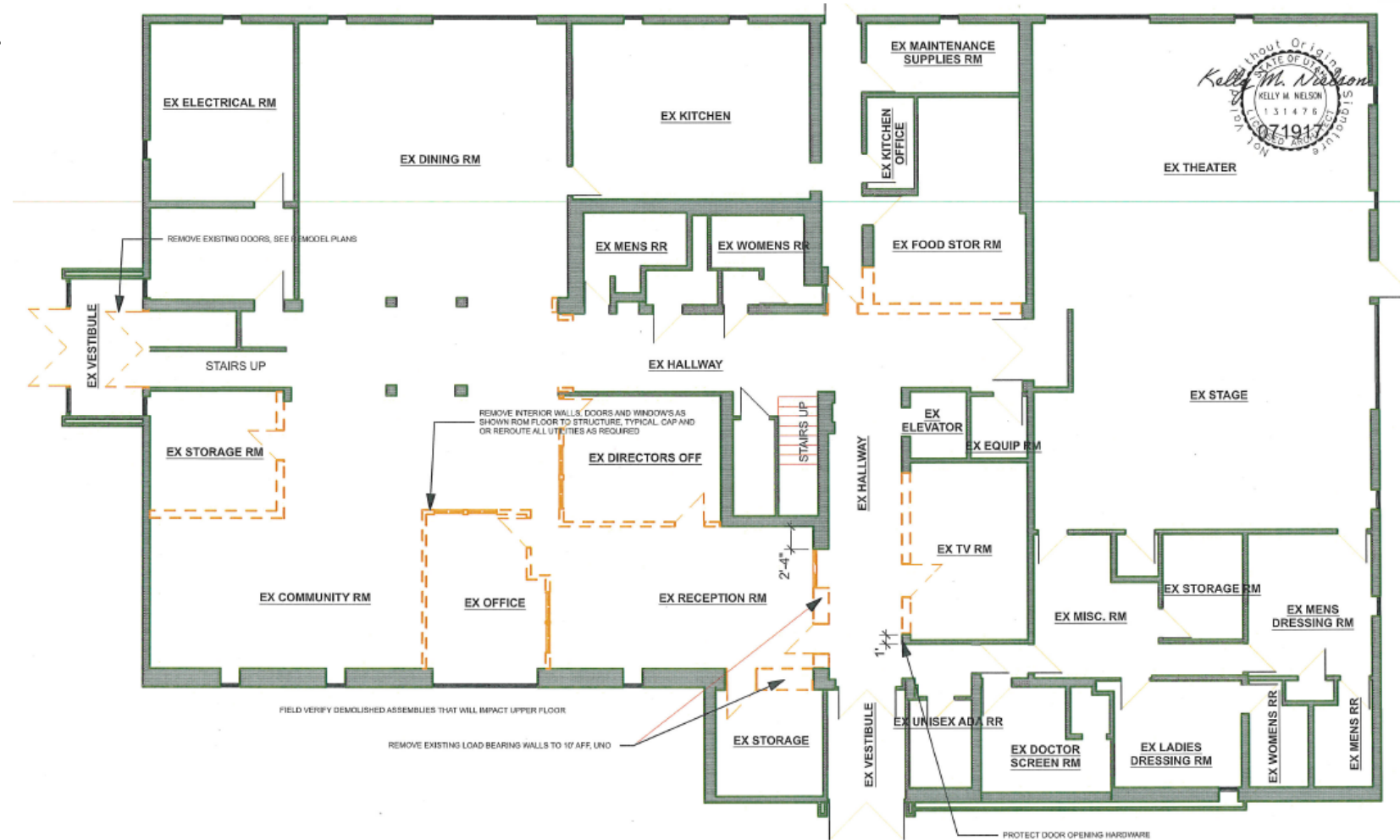
1 GROUND FLOOR DEMOLITION PLAN
