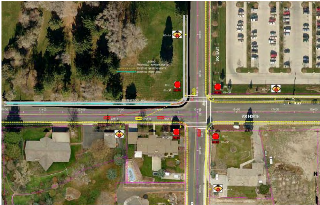
Figure 10: 4-WAY STOP signs with road improvements
