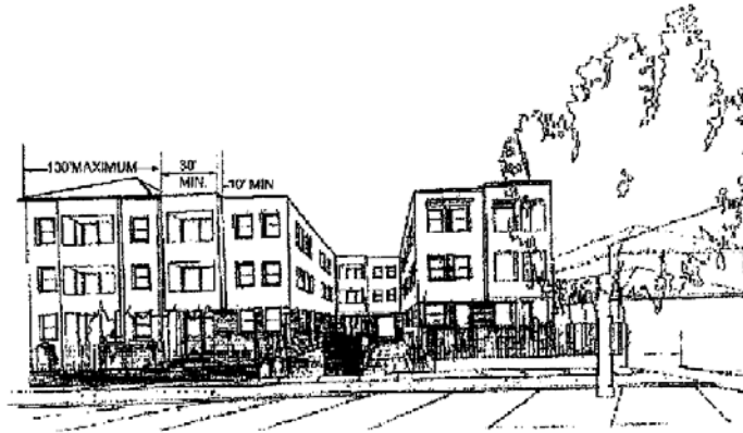
Typical Roofline Breaks
